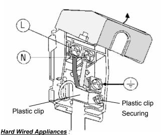
When making the mains supply conductor connections to the terminal block within the terminal box, please ensure that minimum clearances are being maintained between individual conductors and conductors/connectors to the adjacent metal surfaces of the terminal box itself. Where possible add heat shrink sleeves to any bare conductor end/connectors prior to securing.
