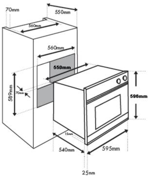
To provide adequate ventilation, there must be an appropriate ventilation opening, the panel to which the oven is fitted should have a gap of at least 70 mm at the rear.
