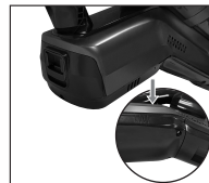
Push the battery pack to lock in position
