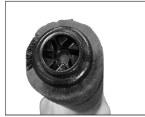
Geared end of roller
