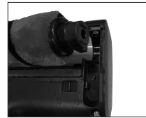
Slide it into the slot on the roller holder
