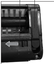
Push the locking tab leftward to unlock
