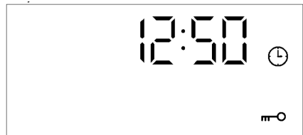
Pic 8: Door lock activated under standby status
